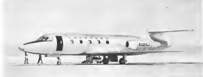
FIRST PROTOTYPE OF CL-329 is powered by two Bristol Olympus 17F turbojets. Production plane will use five GE J85s.
